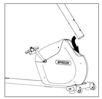
Figure 13: Upright support installation
